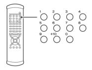
Use the +10 button and 0 through 9 buttons in exactly the same way as when selecting tracks.
